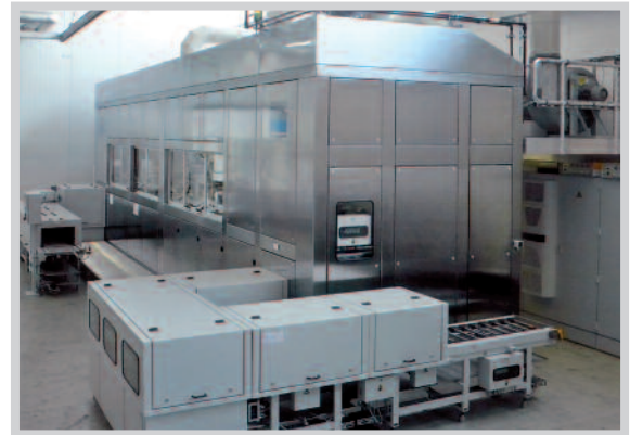
Fully encapsulated cleaning facility in clean room
