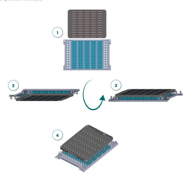
Illustrations: Matching blister (black) to fill the workpiece carrier.
